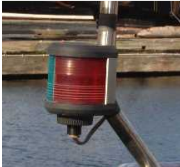
3 A combined lantern plus an all round white light at the masthead.
