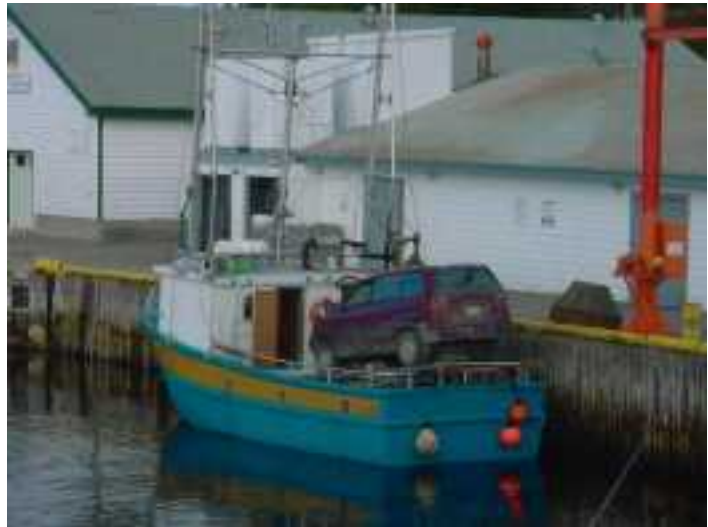
Vessel loading vehicle– vessel stability not within design features. Photograph courtesy Munson Marine
